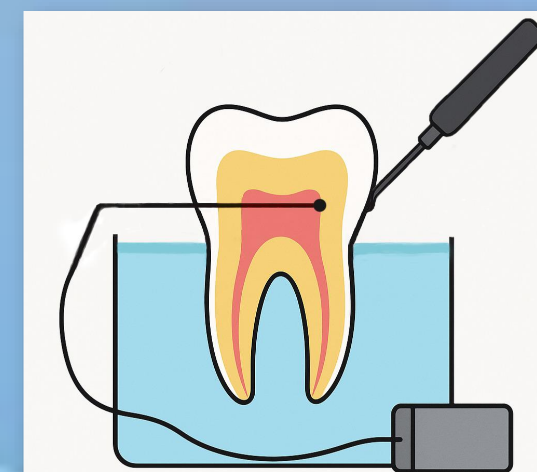
Figure 2. Schematic diagram of placing the probe for measuring the temperature in the chamber and applying heat to the surface of the tooth
