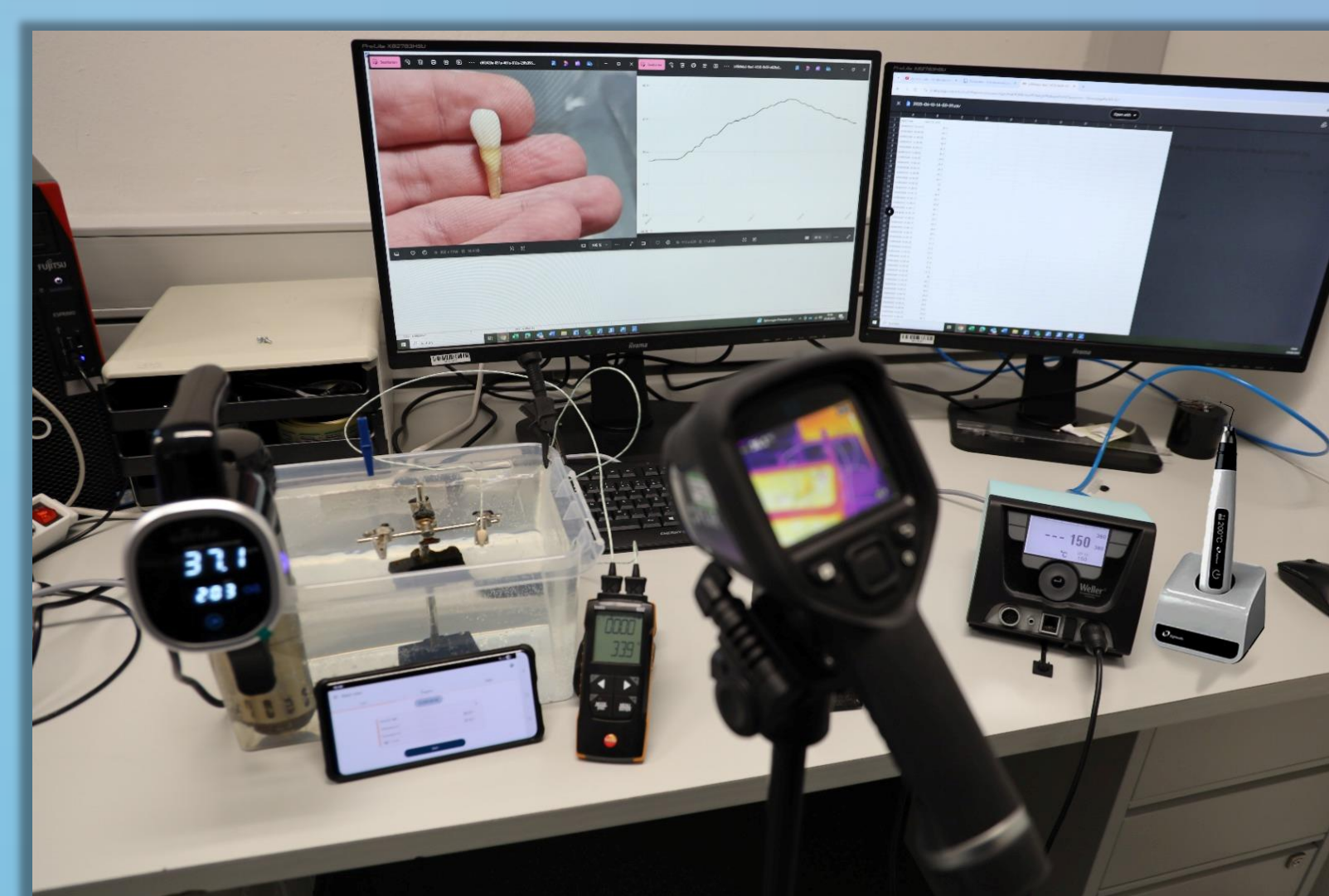
Figure 1. An experimental setup consisting of a tooth submerged in a water bath maintained at 37°C, with a temperature sensor connected to a smartphone application for real-time temperature monitoring
